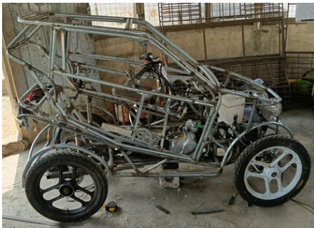
Fig 39: View of the finished frame work
