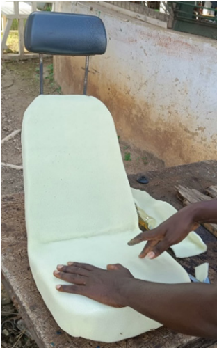
Fig30: Covering the high density with the wrapping foam
