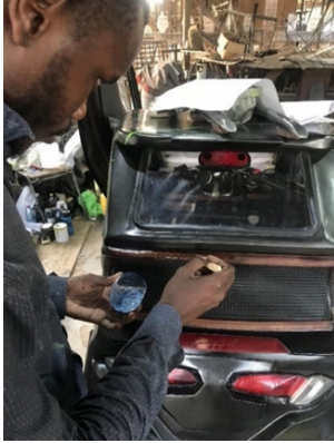
Fig 65: Applying the resin on the wooden part
