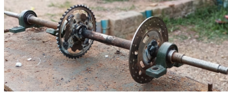
Fig 35: The shaft system with the break disc
