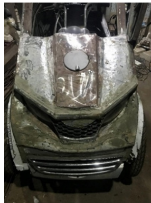
Fig 60: Applying fiber filler
