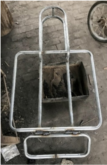
Fig 22: The welded chassis frame
