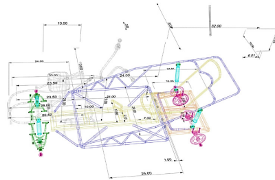
Fig 24: Exploded of suspensions, steer rack, seat
