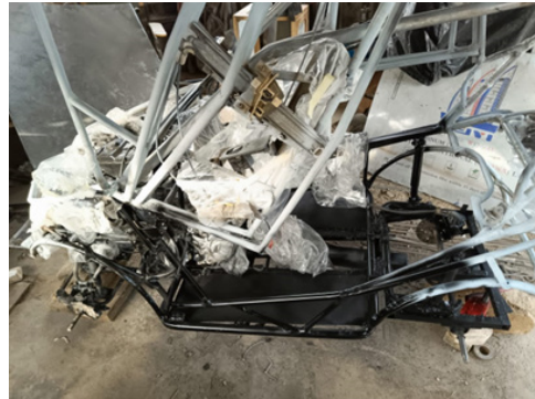
Fig 59: Views of the sprayed frame
