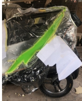
Fig 63: Preparation for painting
