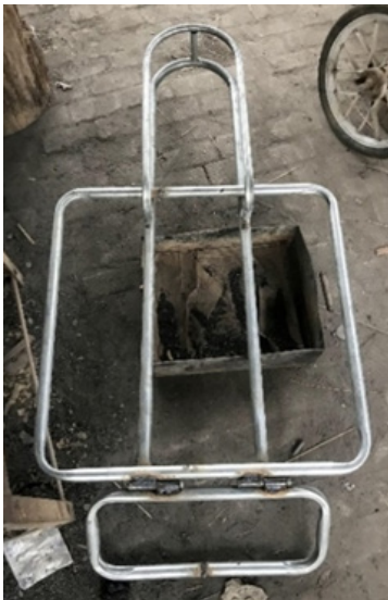
Fig 22: The welded chassis frame
