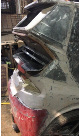
Fig 61: Applied filler on the side of the vehicle
