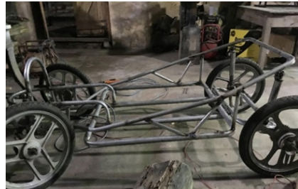
Fig 23: The assembled frame
