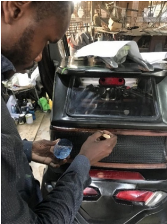
Fig 65: Applying the resin on the wooden part
