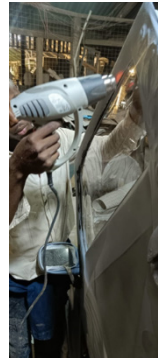
Fig 53: Using the heat gun to bend the fibre glass to conform to the shape of the door
