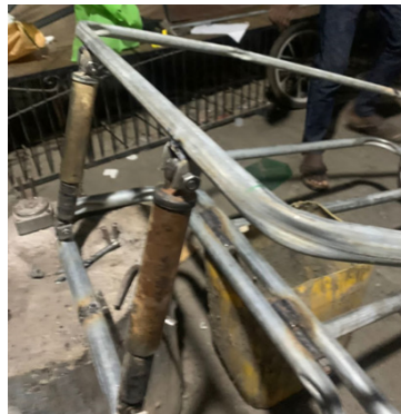
Fig 28: A view of the fixed back suspension
