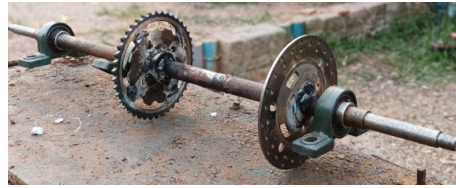
Fig 35: The shaft system with the break disc
