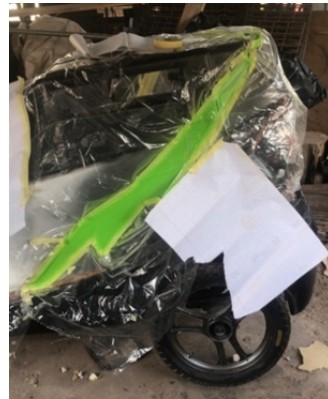
Fig 63: Preparation for painting
