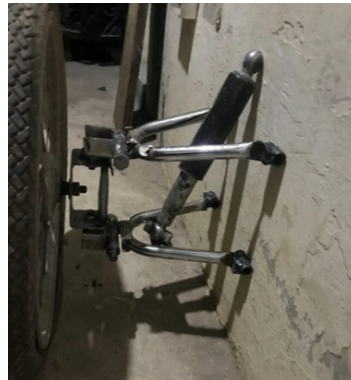
Fig 27: Taking the suspension Alignment measurement.
