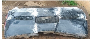
Fig 46: A view of the dried resin for the front bumper
