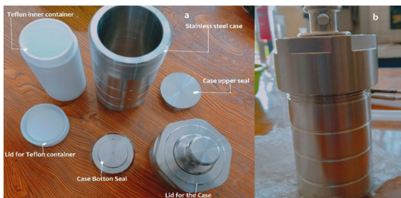
Fig. 2. (a) Parts of the autoclave reactor (b) HTC autoclave reactor
