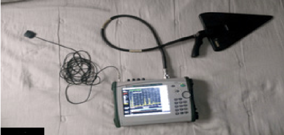
Figure 2: Instrumentation for Electric Field Strength Measurements.
