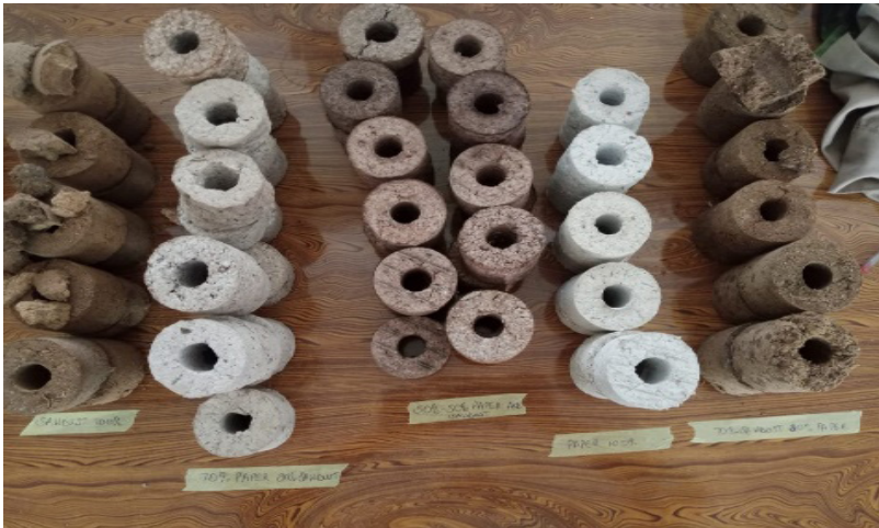
Figure 1: Briquettes formulated from waste paper and sawdust
